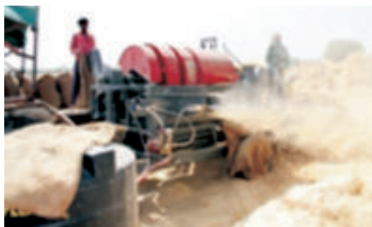
Figure 11: Enrichment of crop residues with Urea: Mechanized urea treatment during threshing operations
